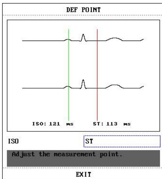
The ISO and ST are the two measurement points in ST segment, both of them can be adjusted.
