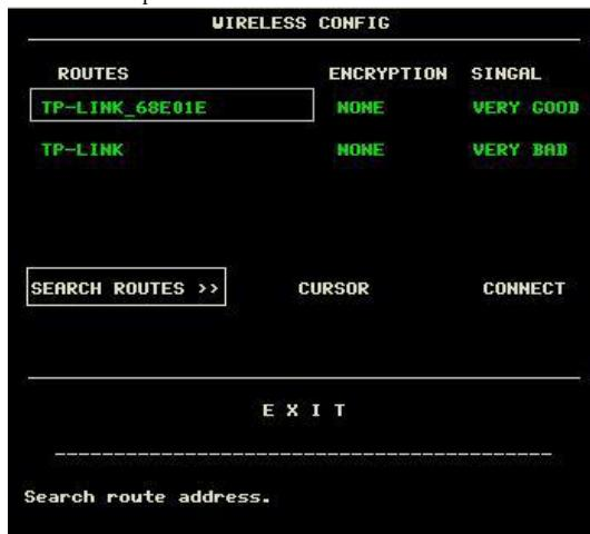
When the network type is CMS, just make sure the connection between the device and the wireless router is successful. (The IP address of the server is 202.114.4.119, the IP address of this monitor and subnet mask are generated by the port number.)
