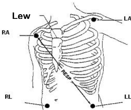
Electrodes Placement (5-lead)
