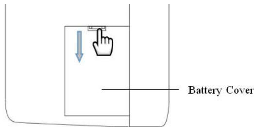
2. Connect the new battery to the connector, place the battery into the slot, then fix the battery compartment
