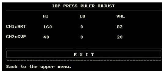
The waveform scale displays in the IBP waveform area, the three dotted lines from top to bottom respectively represent the upper scale, reference scale and lower scale of the waveform, which can be set, the steps are as followings:
