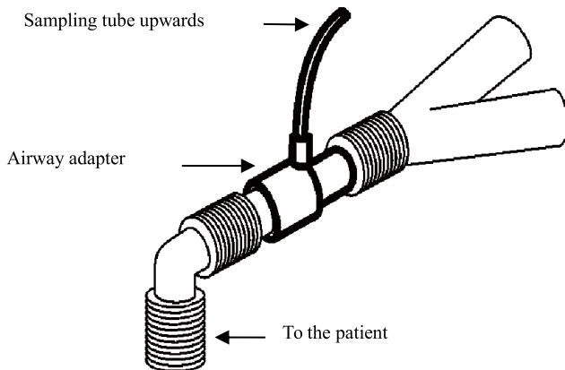
2. For intubated patients with an integrated airway respiration adapter in the breathing circuit: connect the luer male head on the sampling tube to the concave port of the airway adapter.
