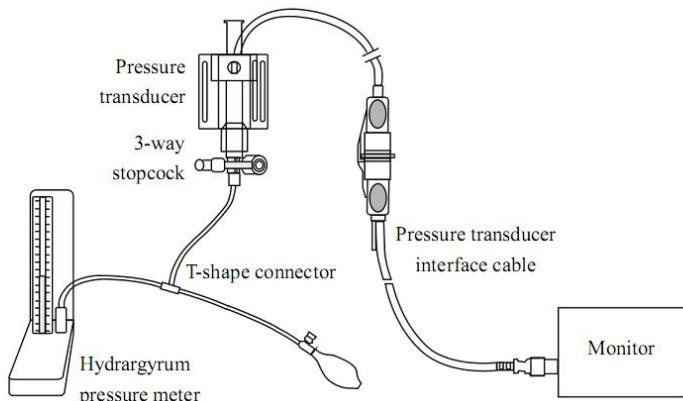
2. The transducer must be vented to atmospheric pressure via the 3-way stopcock.
